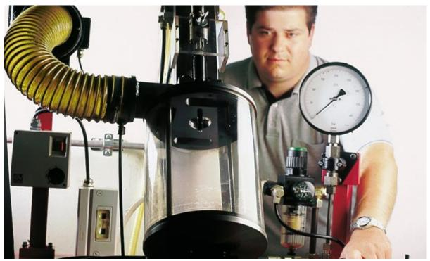
With the reconditioning of injectors, pumps and pressure valves we offer the engine builder an additional service. Parts operating under high pressures, must be machined with the greatest precision and assembled under clinically clean conditions. As part of our policy to ensure the economic use of resources we offer a reconditioning service for these products at planned intervals which have been agreed with our customers.
