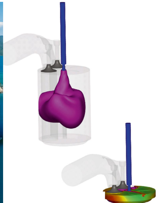
FIGURE 3 CFD injection simulation (upper left) and lambda distribution (© ITAZ)
