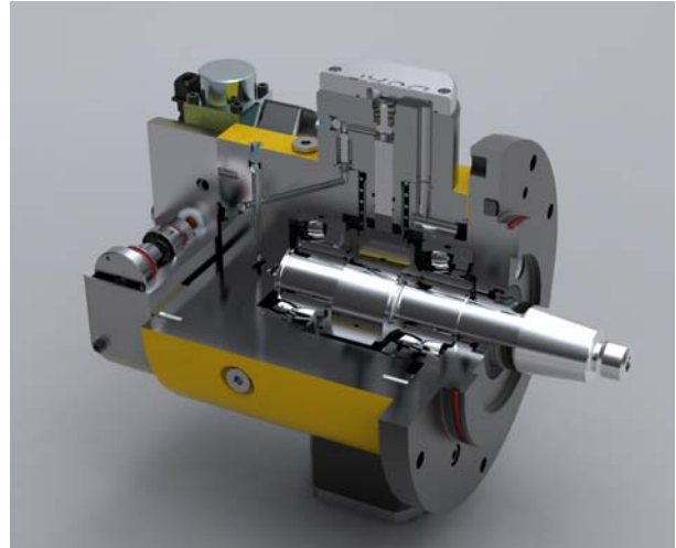
Figure 4 - Cross section of the DUAP 12-DF-2R pump
