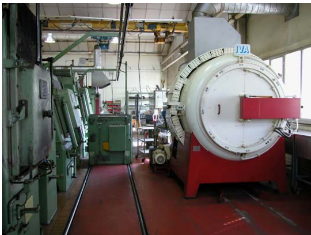
Figure 2 – Tempering furnace in heat treatment shop at DUAP site in Herzogenbuchsee
