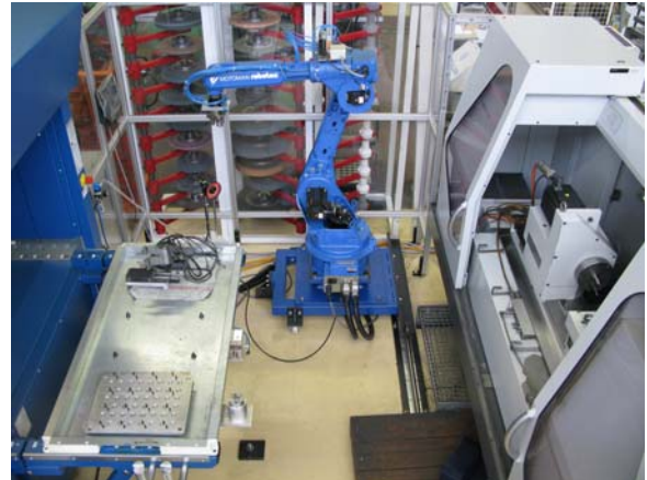
Figure 3 - Cylindrical grinding machine with robot arm for automatised feeding of workpieces
